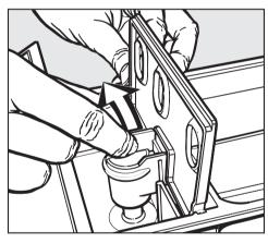
■ Remove the siphon tube from the fabric softener compartment ⊗ and rinse under warm water.
